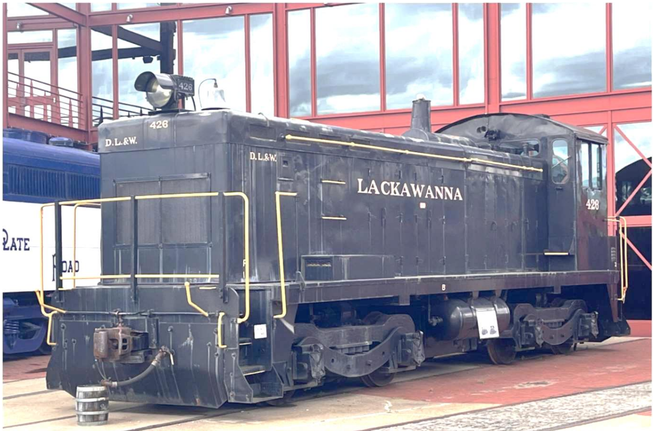
Electromotive Corporation (EMC) 1935 600 HP Pre-Production, Pre-SC Switcher, Originally Powered by a Winton 201-A in-line 8-cylinder Engine. From the Dawn of the Diesel Age.
