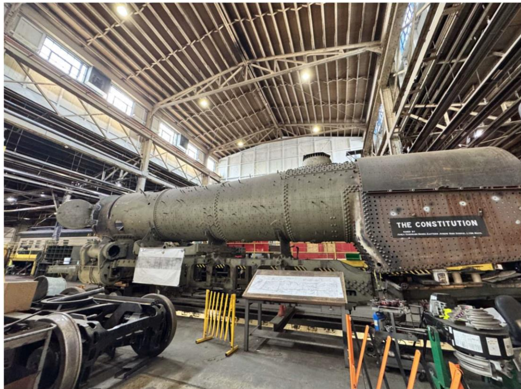
This Boiler Undergoing Testing and Restoration Belongs to Boston and Maine No. 3713 is a 4-6-2 "Heavy Pacific" type steam locomotive built by the Lima Locomotive Works in December 1934
