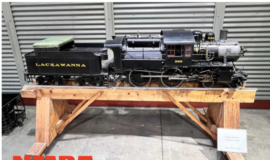
Live Steam Riding Model of Lackawanna Mother Hubbard 4-4-0 American Locomotive #988.
