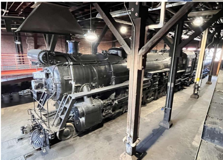
Grand Trunk Western No. 6039, a Class U-1-C 4-8-2 "Mountain-type" Dual-Service Locomotive. Built in June 1925 by the Baldwin Locomotive Works in Eddystone, Pennsylvania.
